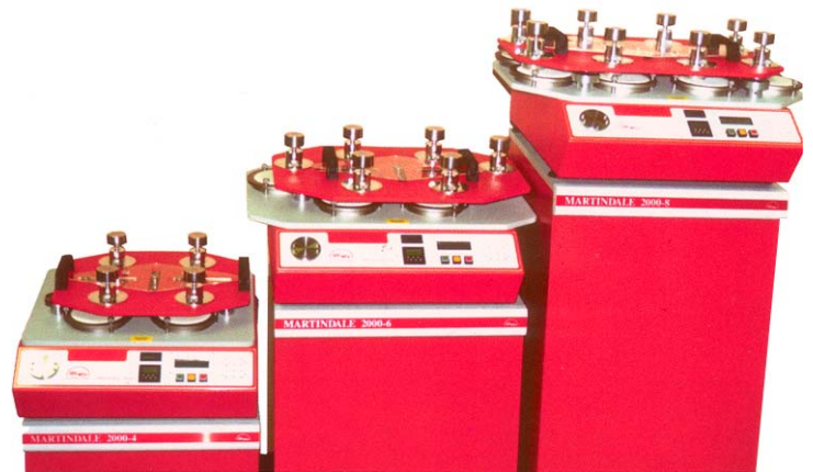
Martindale testers with 4, 6 or 8 test stations
