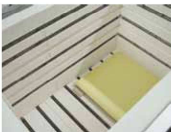
Firing chamber with heating from 5 sides
