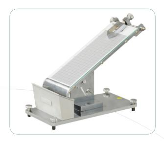
CZY-G is based on the balling method, and the primary adhesive property of adhesive tapes could be obtained by observing adhesive effect occurred immediately after rolling ball and adhesive specimen come into contact.
