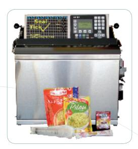
The package integrity tester (P.I.T.) uses a vacuum method to measure the gasleaking from a wide range of flexible pack types and sizes. Items are placed manually into the unit, and the handle is closed to initiate the test sequence. Results are displayed as a Pass or Fail, along with a quantitative measure of the leakage rate.
