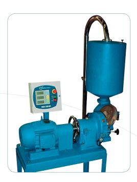
The laboratory disc refiner, type Bauer, is widely used for pilot refining of chemical and semichemical pulps, chips and recycled paper in the quality control and R&D.
