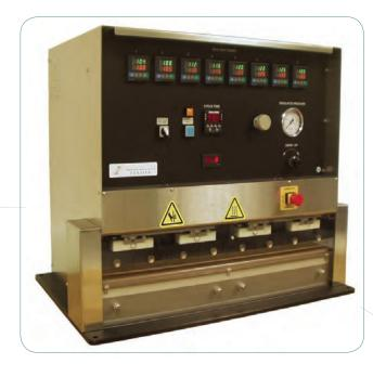
The 24" CeraTek Heat Sealer model features eight temperature zones along the length of the upper heated jaw (each of the eight zones is independently controlled via eight separate temperature controllers). Each zone is 2 7/8" x 1" and there is 1/8" between each zone to minimize the effects of heat transfer from adjacent zones.
