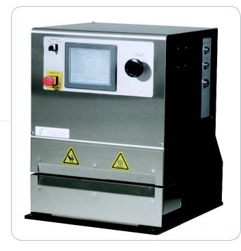
CeraTek P-Series Heat Sealers feature a precision passthru system. The machine design allows both frontto-back and lateral pass-thru capabilities. The cycle is activated with a locking foot switch circuit. Safety features include zero access guarding and an e-stop circuit.
