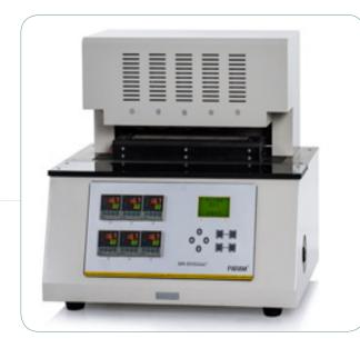
GHS-03 Gradient Heat Seal Tester is professionally designed for the determination of heatsealability of plastic films, composite films, coated paper, and other sealing films under certain sealing speed, pressure and 5 different temperatures. The heatsealability of heat sealing materials would be greatly affected by the factors of melting point, thermal stability, fluidity and thickness. The properest heatsealability parameters could be obtained accurately and efficiently through this instrument.
