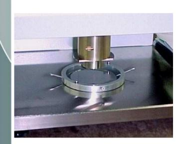
Parallelism: Check variation in flatness between the anvil and pressure foot
