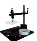
TS-02 closed package test xture in conjunction with an entry system such as the Package- Port<sup>©</sup> system, allows you to test completely sealed exible packages. A variety of probe sizes is available to further customize your test system.
