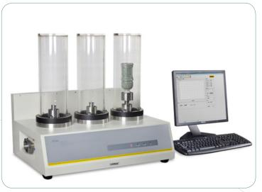
This is based on the differential pressure method, and professionally applicable to the determination of gas transmission rate of finished package containers. Test gases could be air, oxygen, nitrogen, and carbon dioxide, and testable containers include various bottles of carbonated drinks, juice, tea, as well as packages of edible oil, dairy products, washing supplies and metal containers.
