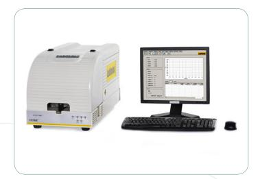
G2/132 is based on the differential pressure method and is professionally applicable to the determination of gas permeability of film specimens. It is equipped with three diffusion cells, which could generate test results of three equivalent specimens at one operation. The testing process conforms to GB, ISO, ASTM and many other international standards.
