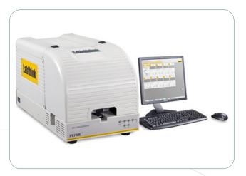
This instrument can be used to measure oxygen transmission rate of film and package specimens. It has three test modes and is applicable to various materials with high, medium and low oxygen permeability. It is also embedded with high precision oxygen sensor, which provides a wide test range of 0.01 ~ 65,000 cm3 /m2 •d and durable service life
