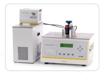
This instrument is professionally applicable to the determination of water vapor transmission rate of plastic films, composite films, high barrier materials, back-sheets, sheeting, aluminum foils, waterproof materials, and other materials used in sanitary and medical industry. By testing the water vapor transmission rate, the technical indexes of materials could be controlled to meet the requirements for production.
