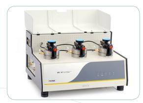
VAC-V2 is based on the differential pressure method, and is professionally applicable to the determination of gas transmission rate as well as solubility coefficient, diffusion coefficient and permeability coefficient of plastic films, composite films, high barrier materials, sheeting, and aluminum foils.
