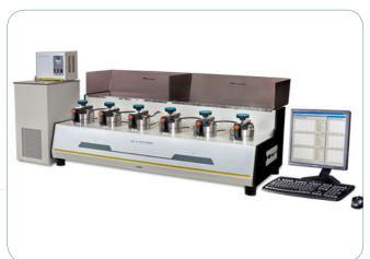
VAC-V3 is based on the differential pressure method, and is professionally applicable to the determination of gas transmission rate as well as solubility coefficient, diffusion coefficient, and permeability coefficient of plastic films, composite films, high barrier materials, sheeting, and aluminum foils.
