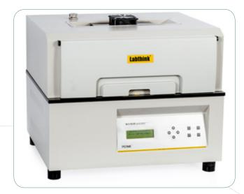
W3/0120 Water Vapor Transmission Rate Tester is based on the cup method, and is professionally applicable to the water vapor transmission rate test of plastic films, composite films, sheets and other materials used in medical and other industry. By testing the water vapor transmission rate, the technical index of the materials could be controlled to meet the requirements for production.
