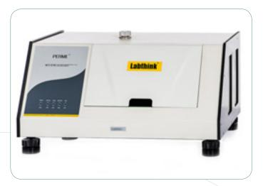
W3/030 Water Vapor Transmission Rate Tester is based on the cup method, and is professionally applicable to the water vapor transmission rate test of plastic films, composite films, sheets and other materials used in medical and construction industry. By testing the water vapor transmission rate, the technical index of the materials could be controlled to meet the requirements for production.
