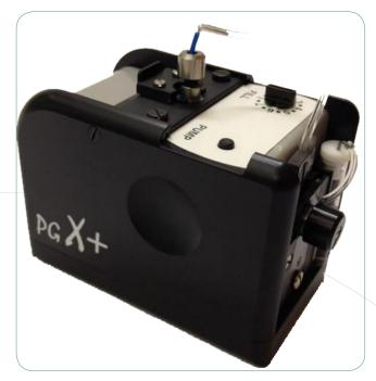
The PGX+ is a compact instrument that measures wetting and absorption on virtually any size or shape sur-face without the need to cut sample strips required by other contact angle testers.
